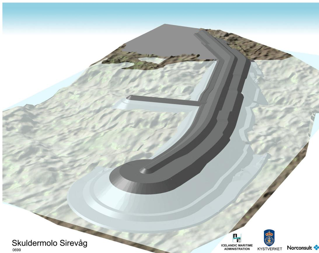
Figure 1. The Sirevåg berm breakwater
