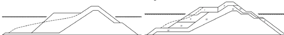
Figure 1. Mass armoured berm breakwater to the left, MA, and Icelandic-type berm breakwater to the right; IC. On both cross sections the expected reshaping is shown with a dotted line.
