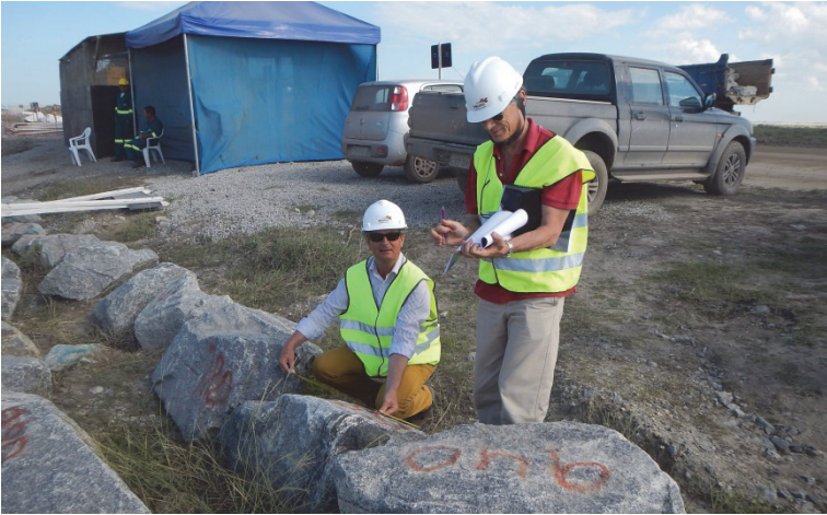
Figure 7.16. Calibration of “three-side method” on known rock masses from 1-6 t.
