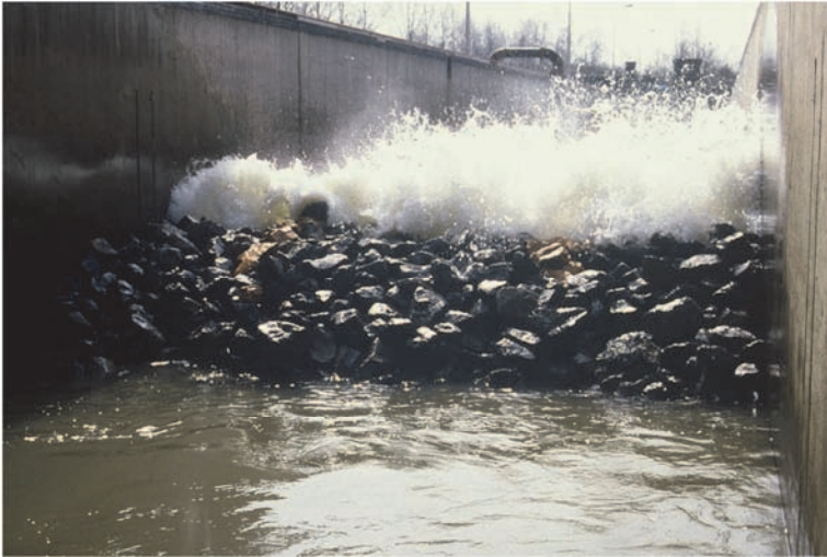
Figure 4.20. A wave breaking on a berm breakwater in the Delta flume of Deltares, giving a transmitted wave height after overtopping.
