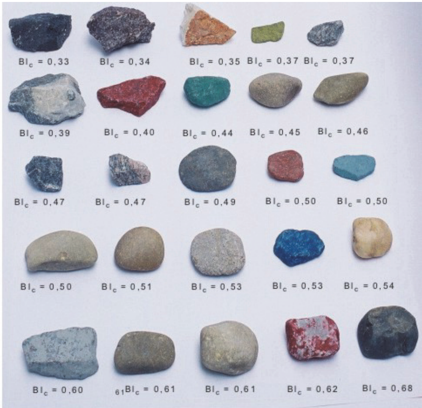
Figure 7.20. Different rock shapes ranked according to their blockiness coefficient BL_c .
