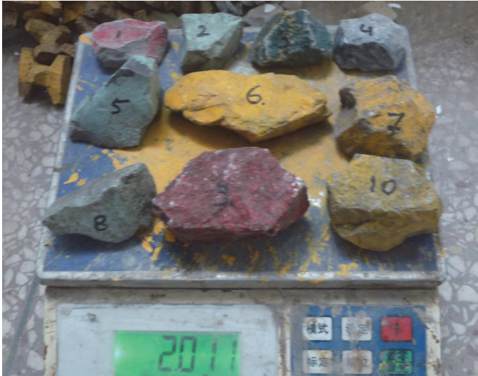
Figure 7.23. Ten stones used to estimate the mass by measuring sides.
