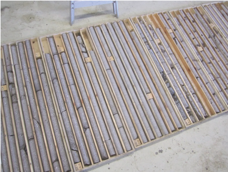
Figure 6.6. Drilled borehole cores which have been analysed for quarry yield prediction of a breakwater project in Husavik, Iceland.
