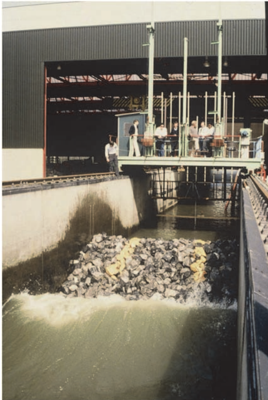
Figure 5.6. Testing a fully reshaping berm breakwater in the Deltaflume (Courtesy Deltares).
