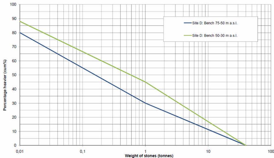
Figure 5. Preliminary bench yield prediction for Quarry Site D, based on the first drilling phase
