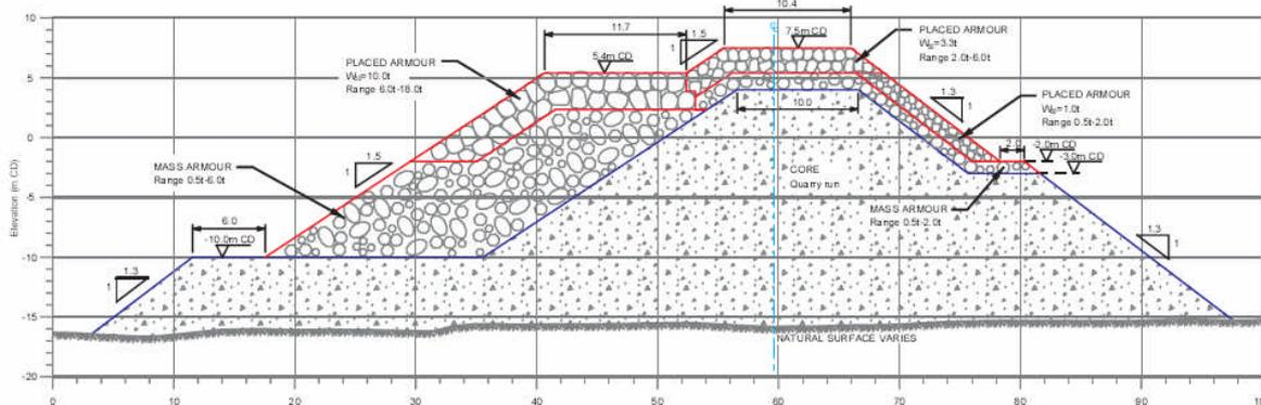
Figure 2. Typical cross section of the Icelandic-type berm breakwater
