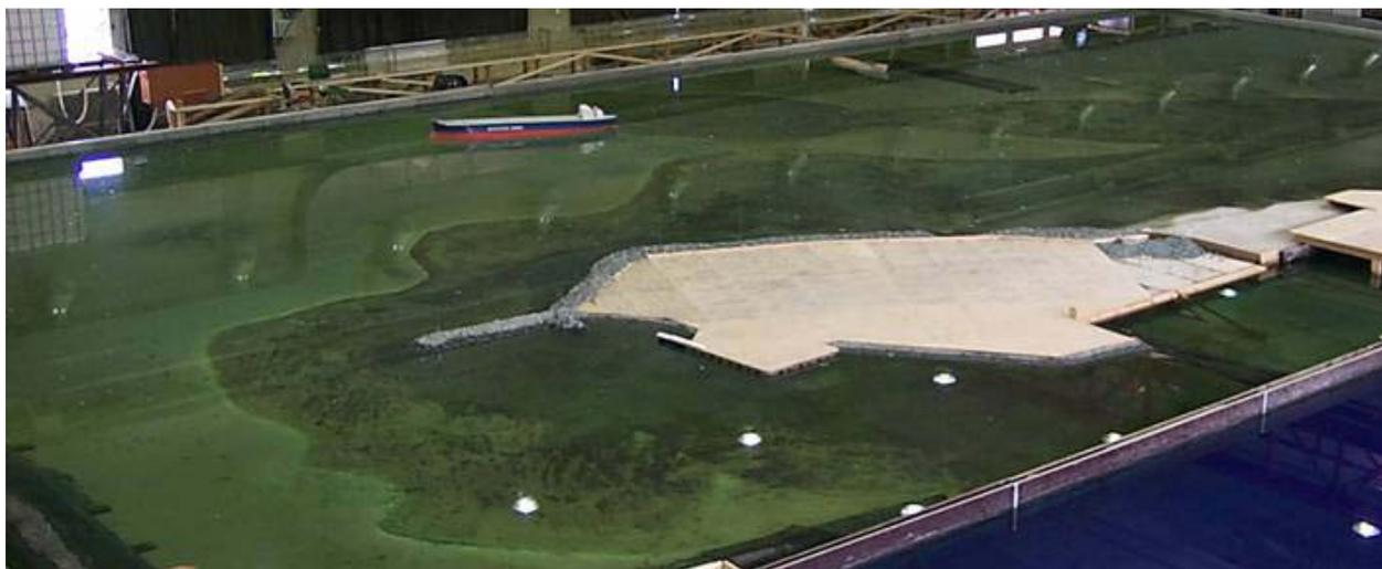
Figure 4 View of physical model of Melkøya. Waves approach from the upper right of the image. The triangular shaped structure in centre front is the Construction Jetty.
