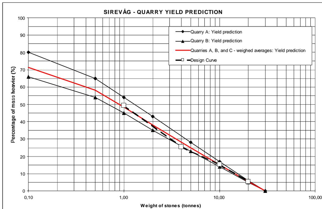
Figure 3. Quarry yield prediction for and design curve for the Sirevåg breakwater.
