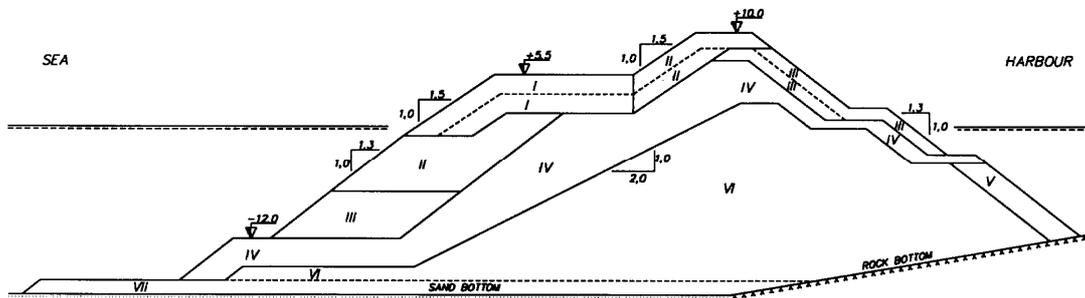
Figure 4. Sirevåg berm breakwater, cross section for the outer part.
