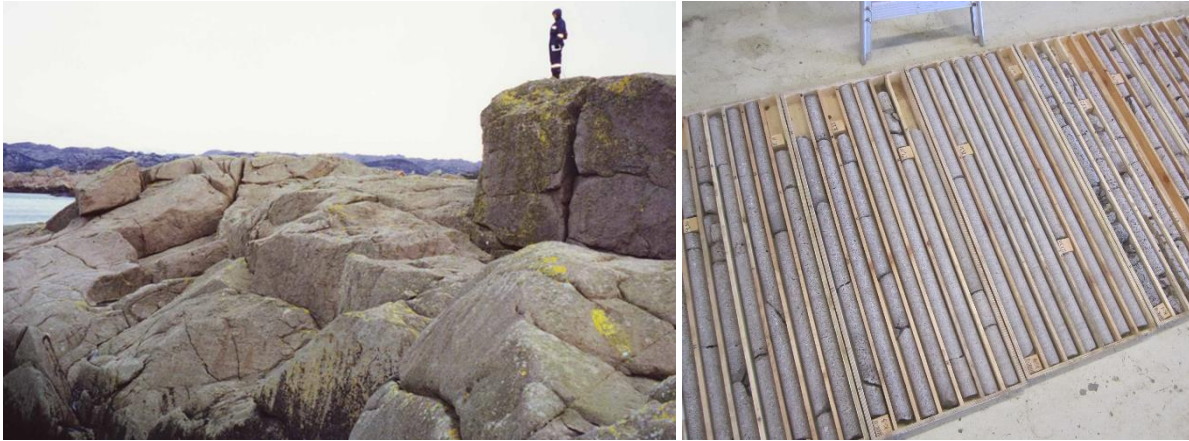
Figure 1: Coarse fracture pattern of the rock for the Sirevåg berm breakwater to left. Drilled cores that have been analysed for quarry yield prediction for a breakwater project in Husavik.
